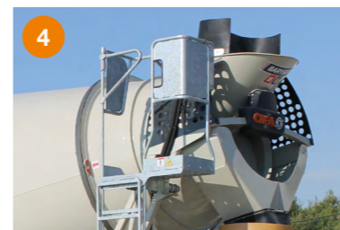
4 Hot galvanized ladder, complies with EN12609
