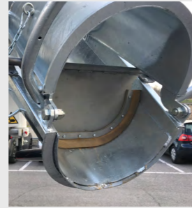
Concrete chute flap.
