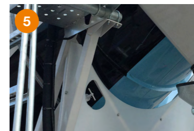
5 Drum safety stop for truck mixer maintenance and plastic back cover.
