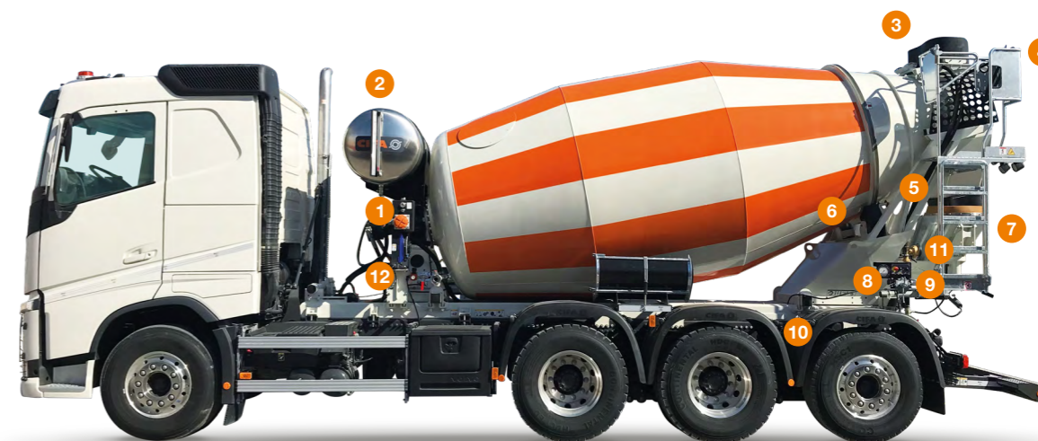
12 Double water inlets. Water can be filled from both right and left side of the truck mixer. Heat exchanger with oil tank. Manometer for concrete consistency.
