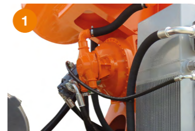
1 Water pump installed on the reducer.
