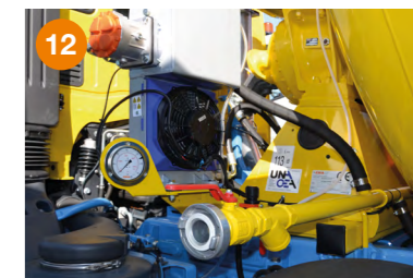
12 Double water inlets. Water can be filled from both right and left side of the truck mixer. Heat exchanger with oil tank. Manometer for concrete consistency.
