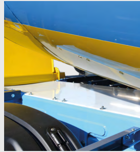
Cover protection under the drum.
